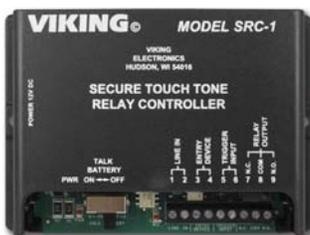
C-250 software has been updated to provide a short delay to allow for keyless entry. The SRC-1 provides the keyless entry capability and stores up to (32) one to six digit keyless entry codes. The user dials a “#” plus a valid keyless entry code to let themselves in. The C-250 must have a part number (“P/N”) of 262258B in order to have this capability.
