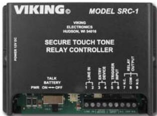
Viking engineers have created SP437 based on the C-250 that provides a short delay to allow for keyless entry. The SRC-1 provides the keyless entry capability and stores up to (32) one to six digit keyless entry codes. The user dials a “#” plus a valid keyless entry code to let themselves in.
