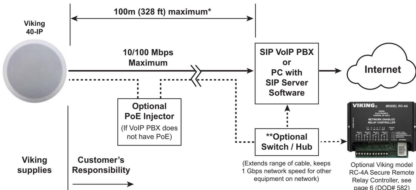
\* **Note:** A PoE extender can be used for an additional 100 meters per extender. For longer runs (up to 2 km / 1.2 miles) a ethernet to fiber media converter can be used.
