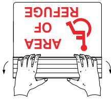
Fig. 1 Opening Aluminum housing cover
