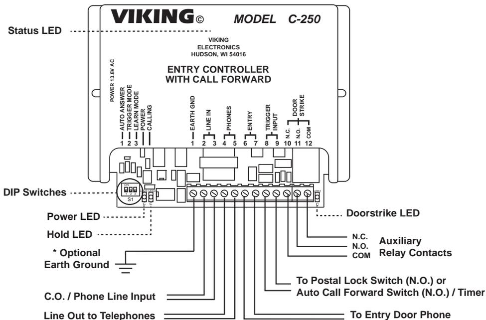
\* **Note:** To increase surge protection, fasten a wire from the screw terminal to Earth Ground (grounding rod, water pipe, etc.)
