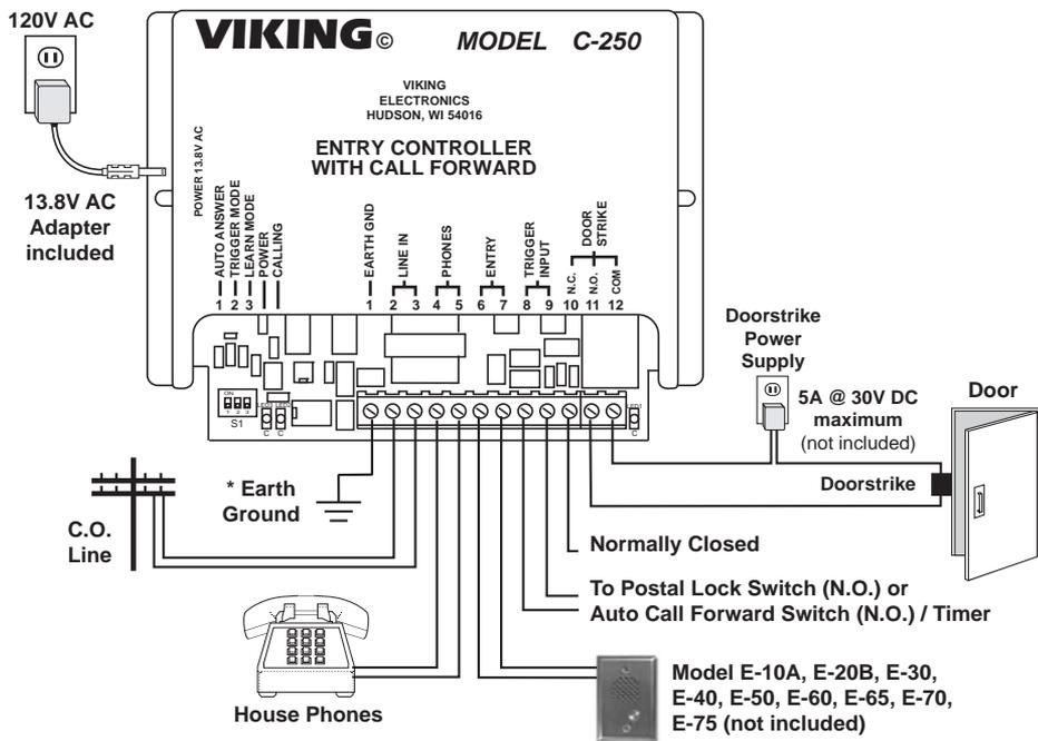
\* **Note:** To increase surge protection, fasten a wire from the screw terminal to Earth Ground (grounding rod, water pipe, etc.)
