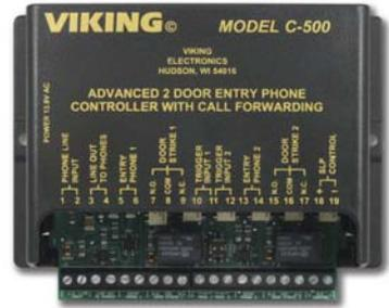
The **C-500** allows up to 6 permanent keyless entry codes, 2 "one time use" entry codes and 1 toggle entry code for each door. The **C-500** provides optional entry phone distinctive ring, two trigger inputs for "Request to Exit" and field programmable Caller ID or beep tones when answered to indicate which door is activated.
