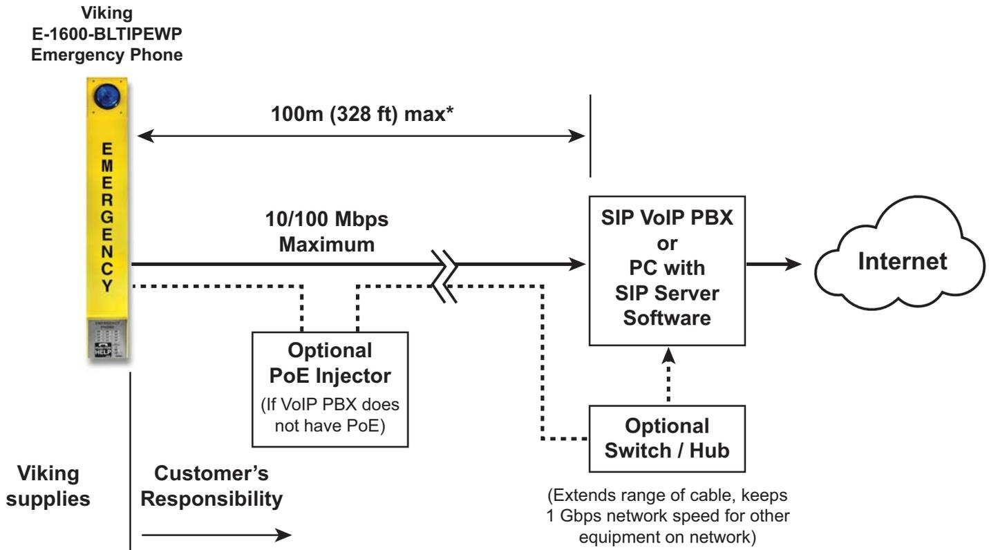
\* **Note:** A PoE extender can be used for an additional 100 meters per extender. For longer runs (up to 2 km / 1.2 miles) a ethernet to fiber media converter can be used.
