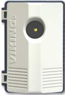
This auxiliary electronic ringer operates on any analog line that provides a minimum of 40 volts 20-30 Hz AC ring voltage. Nominal 3 KHz warble provides adequate volume for business offices. The **LPR-1** can be connected via screw terminals or modular RJ-11 jack. A volume control and a 7 foot modular cord are provided. No power supply is required.
