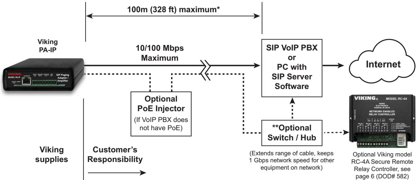
\* **Note:** A PoE extender can be used for an additional 100 meters per extender. For longer runs (up to 2 km / 1.2 miles) a ethernet to fiber media converter can be used.
