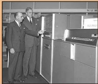
IBM created the first calculating machine to use solid-state transistors instead of tubes. The end result was a 2,000 transistor calculator no smaller in size and no faster in speed. Transistors were cheaper, took less power and created less heat.
