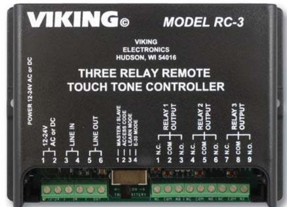
The RC-3 enables a standard touch tone phone to control up to 3 maintained ON, maintained OFF, or momentary relay contacts from a remote location. The RC-3 is fully user programmable and uses non-volatile memory. Up to three RC-3's can be daisy chained on the same line to control up to nine relays.
