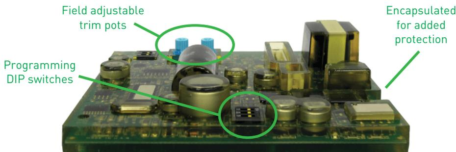
Finally we surround the entire board in a flexible urethane or thermoplastic encapsulating material (shown above), leaving the internally sealed field adjustable trim pots and DIP switches accessible. This special material allows the circuit board and its components to expand and contract, while maintaining weather resistance. To protect the wire connections, we include connectors filled with anti-corrosive sealing gel.
