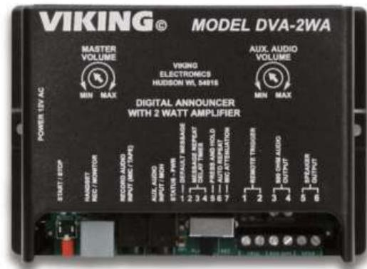
The **DVA-2WA** features non-volatile memory and eliminates the need for batteries or costly built in tape decks. This provides the convenience of recording at the shop or professional studio and then shipping to the installation site.
