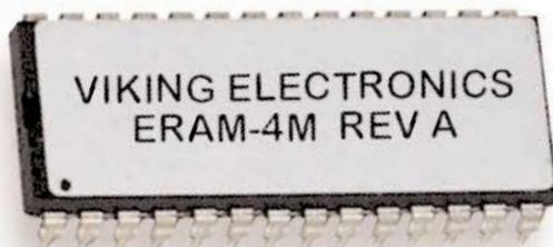
The ERAM-4M Memory Expansion Kit is designed to expand the voice record memory of the AES-2000 using non-volatile memory.
