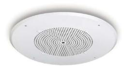
The Viking model **SA-1S** is an 8 inch paging speaker that has a built in 1.5 watt power amplifier, an infrared remote control detector, and an integrated digital volume control, all built into an attractive off-white grill for flush mounting in office ceilings. The **SA-1S** self amplified paging speaker uses a proprietary two wire protocol in which both 40 volts DC power and audio are combined on the
