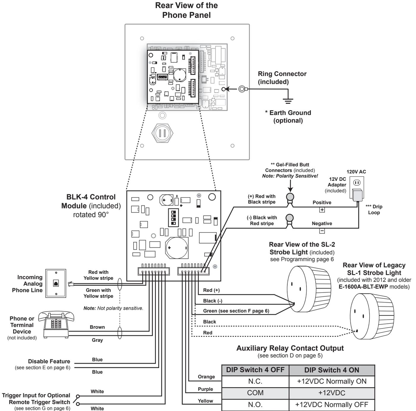
\* **Note:** To increase surge protection, loosen the PCB mounting screw labeled ⊕ (as shown) and fasten a wire with ring connector (included) from the mounting screw to Earth Ground (grounding rod, water pipe, etc.)
